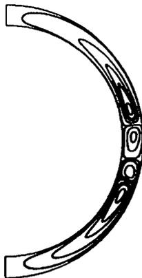
Figure 14. Streamline of the asymmetric 1-vortex flow mode,  $\sigma = 0.154$ ,  $Re = 1500$
